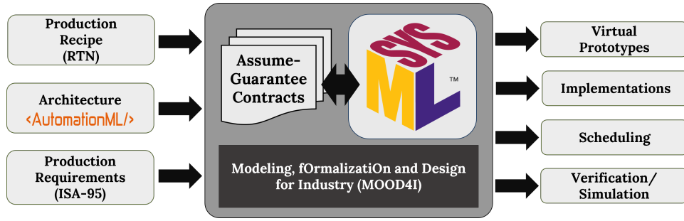
Figure 1: Overview of the conceptual flow proposed by the Modeling, Formalization & Design for Industry (MOOD4I) framework.
